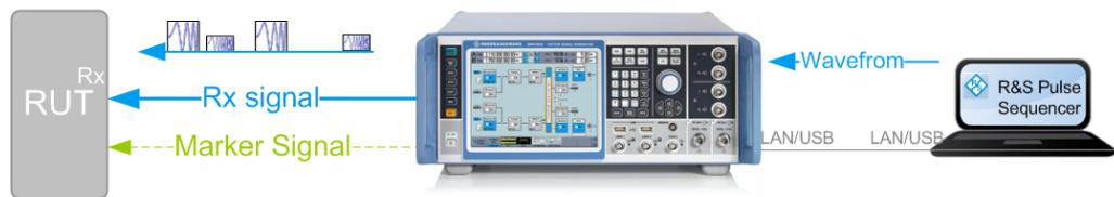
Figure 3-3: Radar echo generation with R&S SMW and ARB-based radar signals created by R&S Pulse Sequencer
